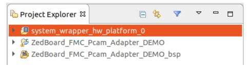
Right Click on system wrapper hardware platform  $\rightarrow$  Change Hardware Platform Specification  $\rightarrow$  Click Yes in the Warning window  $\rightarrow$  Enter the path to the exported hardware location  $\rightarrow$  Click OK.
